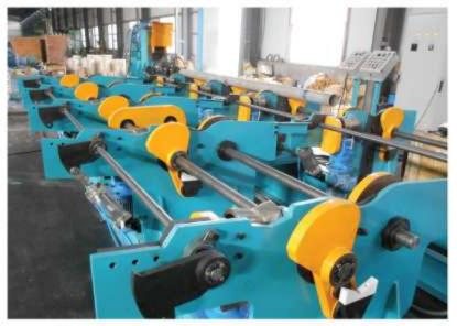
**SMACO** pipe threading machine are fully automatic for both end pipe threading, designed for taper and straight thread to meet various international thread specification, BS, ASTM, ISO etc.
