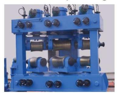
**SMACO** pipe straightening machine are fully automatic with entry and exit conveyor. Heavy duty construction to ensure rigidity of machine during straightening operation.
