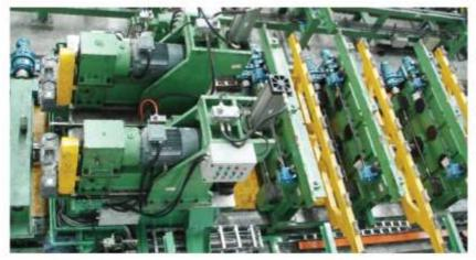
**SMACO** pipe end facing and chamfering machine are fully automatic for both end pipe facing of carbon steel pipe, API pipe, stainless steel pipe and large diameter spiral welded pipe. Standard machine with 2 facing head and high production system with 4 facing head for 2 pipe end facing in one cycle.
