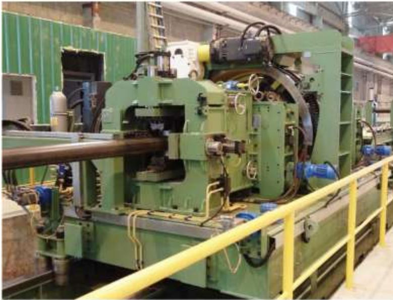
**SMACO** cold saw flying cut-off machine is a high performance cut-off for tube mill line. Available with:
